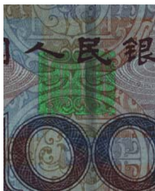
WIDE-BAND VISUALIZATION OF "ANTI-STOKES INKS"
