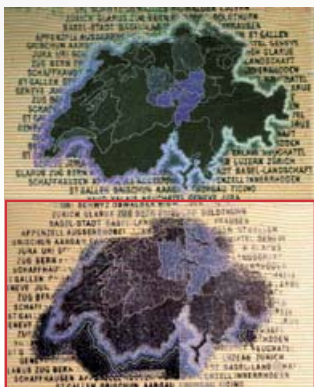
OVI OPTICAL VARIABLE INK ABOVE: ORIGINAL BELOW: FORGERY
