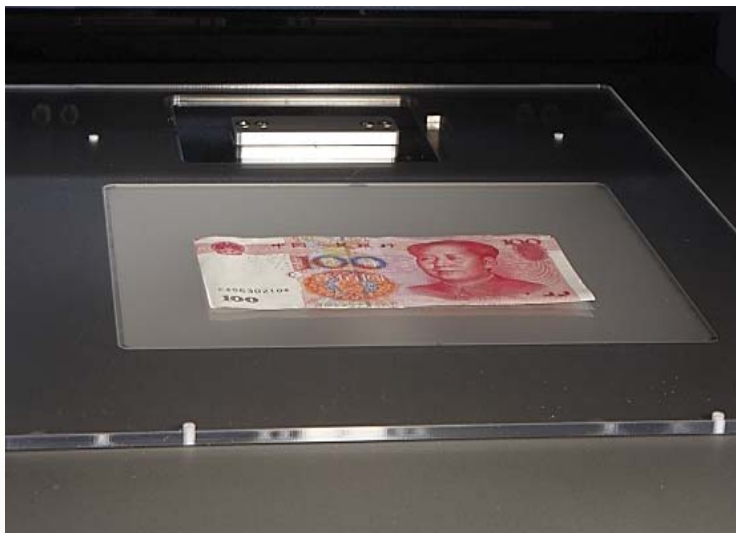
MOTORIZED X/Y TRANSLATION STAGE for optimized positioning of documents
