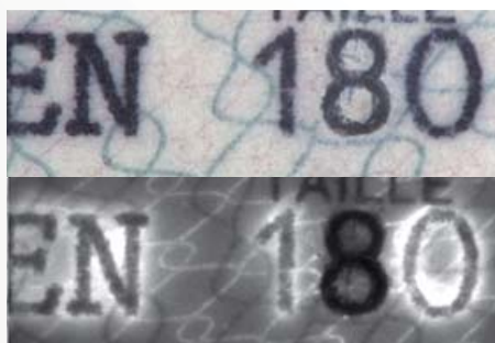
IR LUMINESCENCE INVESTIGATION TOOLS TO DIFFERENTIATE PRINTING INKS
