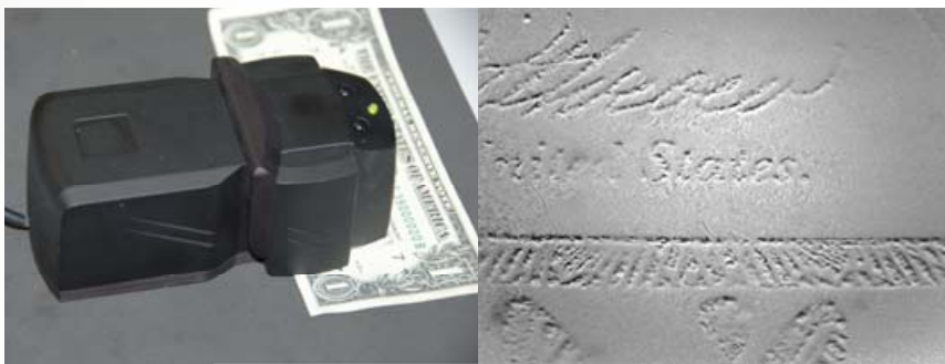
MAGNETIC INK DETECTOR used to visualize magnetic ink in documents
