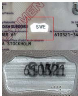
MULTIPLE LASER IMAGE (MLI) VISUALIZATION WITH SIDE LIGHT
